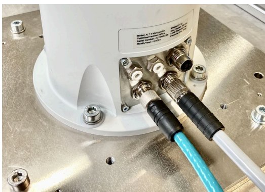
Connecting the manipulator and the controller.
